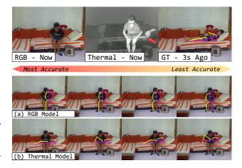
Figure 6. **Importance of thermal imaging.** In this example, it is hard to infer the person's past action through the RGB image. With the thermal image, however, one can easily and reliably infer that the person was lying on the couch.
