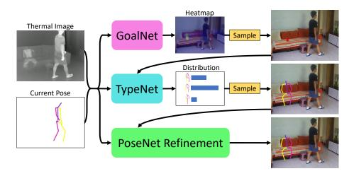
Figure 4. **Overview of our pipeline.** Given a thermal image and an estimated human pose as input, GoalNet first predicts the distribution of the person's location 3 seconds ago and samples one from it. Then, TypeNet predicts pose type distribution and samples one pose from them. Finally, PoseNet refines the pose to match the input observation better. The RGB images are for visualization purposes only.
