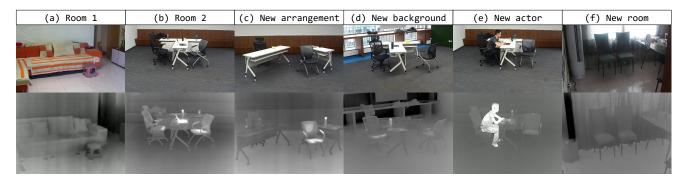
Figure 9. Generalization to new environment: Our training data is collected from two rooms: (a) Room 1 and (b) Room 2. To verify whether our model can generalize to new environment without overfitting, during evaluation we (c) rearrange the object layouts, (d) switch the background, (e) replace the actor, and even (f) test on a complete different room.
