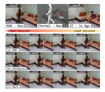
Figure 5. **Comparison against baselines.** We sort the predictions of each approach based on MPJPE and show the 1st, 5th, 10th, and 20th poses from left to right. KNN fails to infer where the person was. Hourglass is able to locate where the person was, but their predictions do not comply with the affordance of the scene. Our method, in contrast, produces reasonable and accurate estimates.
