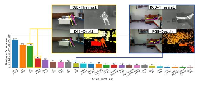
Figure 3. Statistics of our Thermal Indoor Motion (Thermal-IM) dataset. Our dataset comprises 783 synchronized RGB-Thermal and RGB- Depth video clips, with 24 types of human-object interactions. We also provide estimated 2D and 3D human poses in each frame.
