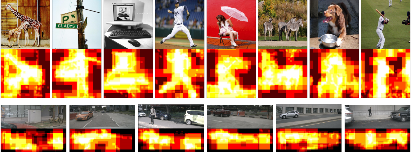
Figure 5. SparseViT effectively prunes irrelevant background windows while retaining informative foreground windows. Each window’s color corresponds to the number of layers it is executed. Brighter colors indicate that the model has executed the window in more layers.
